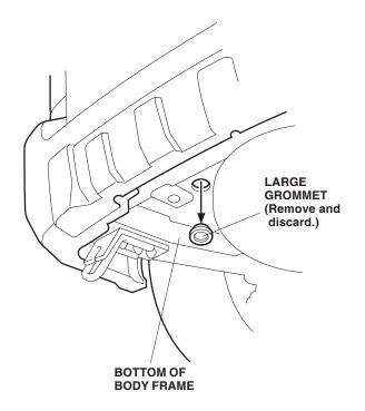
6. Inside the vehicle, locate the grommet on the body panel. Remove and discard the grommet from the body panel.
