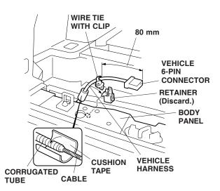
9. Attach one wire tie with clip to the vehicle harness in the area shown. Wrap one cushion tape around the joint section between the corrugated tube of the vehicle harness and cable.
