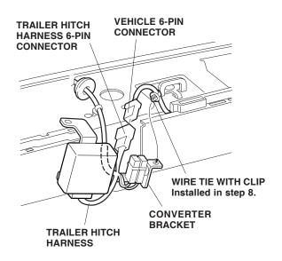
23. Fold the rear cargo box down, and position the converter bracket between the body panel and rear cargo box. Push the clip on the trailer hitch harness 6-pin connector into the body hole where the retainer was removed.
