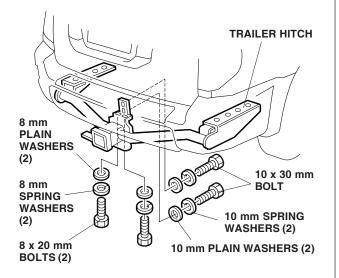
35. Torque the trailer hitch mounting bolts in this order:
