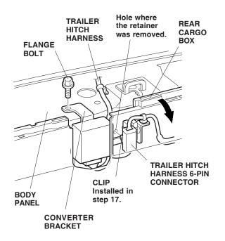
24. Align the hole in the converter bracket with the hole in the body panel and install the flange bolt.
