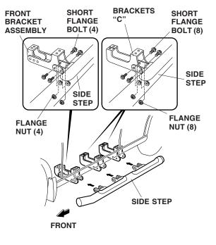
Adjust the location of the left side step so that even clearance is obtained between the side step and body, then tighten the long flange bolts you installed in step 3. Torque the long flange bolts to 27 N⋅m (20 lb-ft)
