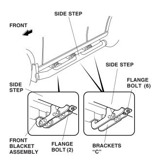
9. Repeat steps 2 through 8 to install the side step on the right side of the vehicle.
