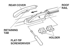
2. Insert two holders in the groove of the roof rail.
