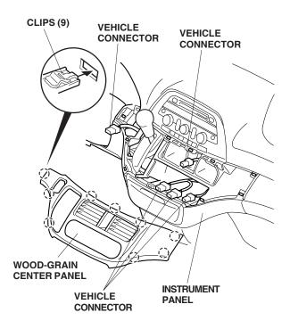
6. Remove the driver's dashboard switch panel (four clips), and unplug the vehicle connectors.
