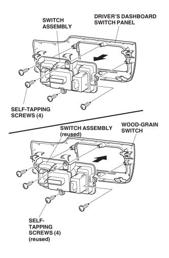
8. Plug in the vehicle connectors, and install the wood-grain switch panel.
