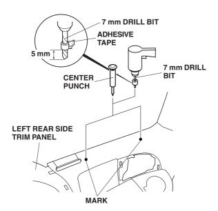
Reinstall the left rear sunshade on the left rear side trim panel, and align the brackets from the left rear sunshade with the holes you drilled.
