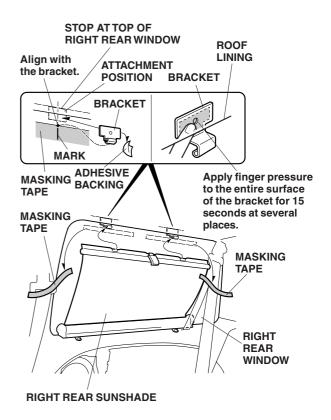
25. Remove the adhesive backing from one of the brackets, and attach the bracket to the top of the right rear window between the marks on the masking tape. Apply finger pressure to the bracket for 15 seconds to allow the tape to adhere to the glass. Install the other bracket the same way. Remove the masking tape from the window.
