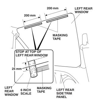
11. Pull up the left rear sunshade. Align the two cutouts in the left rear sunshade with the two strips of masking tape attached to the rear window. Using a felt-tip pen, mark the top of the masking tape at each side of cutout in the rear sunshade. Roll down the left rear sunshade.
