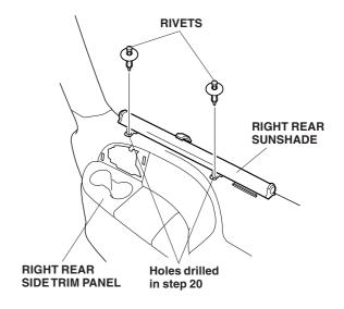
21. Secure the rear sunshade to the rear trim panel using two rivets from the kit, then reinstall the rear trim panel.
