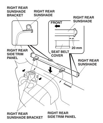
18. Using a felt-tip pen, mark the right rear side trim through the center of each bracket hole. Remove the rear sunshade.
