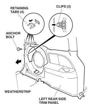
4. Remove the left speaker cover (two clips and three retaining tabs).
