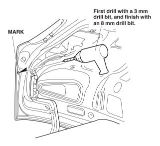
7. Mark the trunk lid stopper with a felt-tip pen, then turn it to the counterclockwise to remove it.
