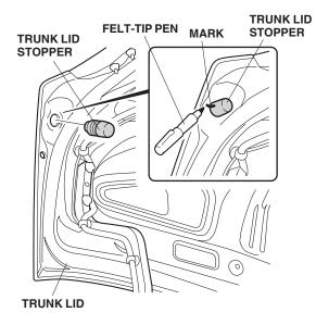
8. Close the trunk lid. Position the template, printed side up, at the left (driver's side) edge of the trunk lid. Align the front hole in the template with the hole in the trunk lid. Using a felt-tip pen, mark the trunk lid as indicated on the template (two marks on the left side).
