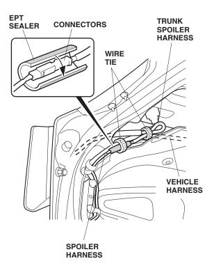
34. Make loops in the trunk spoiler harness, then secure the trunk spoiler harness and spoiler harness to the vehicle harness with the two wire ties as shown.
