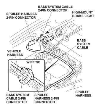
26. Gently pull down the right trunk panel, and locate the clip on the vehicle harness attached to the rear metal shelf. Align the green tape on the spoiler harness with the clip on the vehicle harness, and secure the spoiler harness to the vehicle harness with one wire tie in that area.
