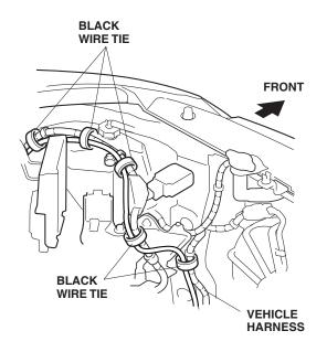
20. Route the heater harness on the inside of the bumper opening and secure it to the grille with two black wire ties.
