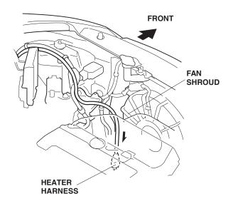
18. Secure the wire tie with clip, (installed on the heater harness in step 10) to the vehicle frame, and route the heater harness to the front bumper opening.
