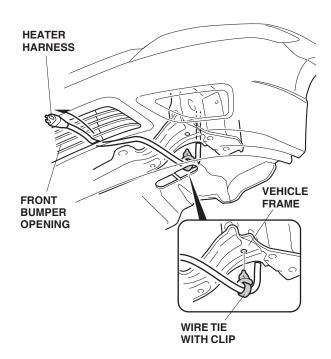
19. Secure the heater harness to the vehicle harness using five black wire ties.
