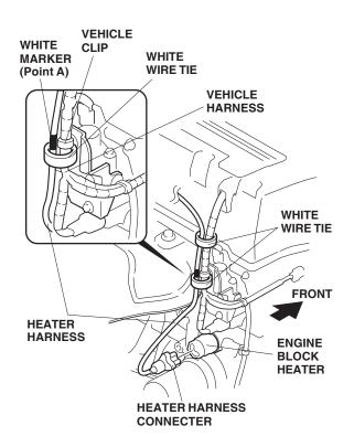
14. Secure the heater harness to the vehicle harness with one white wire tie at the marked point A. Secure the heater harness to the vehicle harness using a white wire tie above the marked point A. 15. Secure the heater harness to the vehicle harness with one black wire tie at the marked point B.
