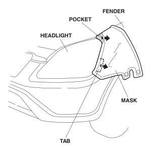
Pull the rear edge of the mask toward the wheelwell, smooth out any wrinkles, and attach the snaps on the mask to the snap-screws on the fender.
