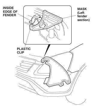
9. Slip the pocket over the upper corner of the fender. Insert the tab between the headlight and the fender.
