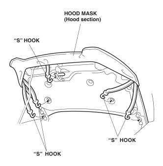
3. Secure the mask by hooking the four "S" hooks to the holes in the back of the hood.
