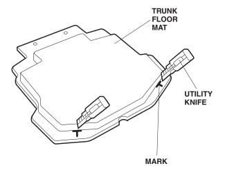
14. Install the four hooks B and washers in the holes in the floor panel, then reinstall the trunk floor mat. Feel the centers of the two front hooks by touching the surface of the trunk floor mat and mark the mat with a felt-tip pen.
