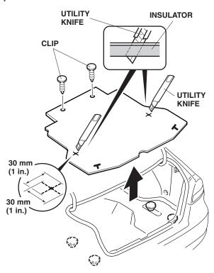
16. Using a tape measure and a felt-tip pen, measure and mark the insulator just behind the two "+" cuts made in step 15 as shown. Cut out the marked areas from the insulator with a utility knife.
