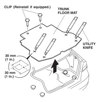
Check the back of the trunk floor mat. If the trunk floor mat has an insulator, continue with step 12; otherwise, go to step 17.
