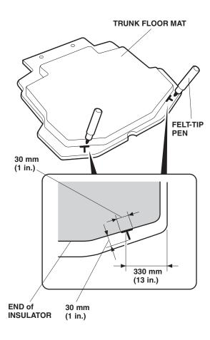
13. Using a utility knife, make a "T" cut in the trunk floor mat at each of the two marks you just made.
