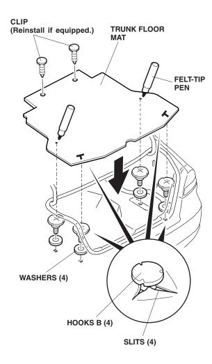
15. Remove the trunk floor mat and make a "+" cut in the trunk floor mat at each of the two marks you just made.
