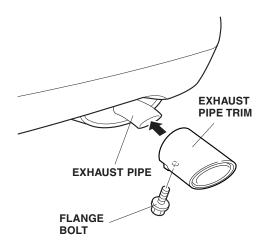
With the flange bolt on the bottom, facing down, slide the exhaust pipe trim onto the exhaust pipe until it bottoms.
