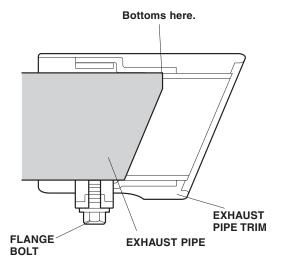
3. While pushing the exhaust pipe trim firmly against the exhaust pipe, tighten the flange bolt.
