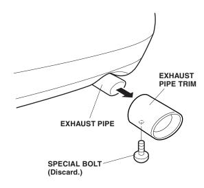
Partially thread the special bolt supplied into the new exhaust pipe trim.
